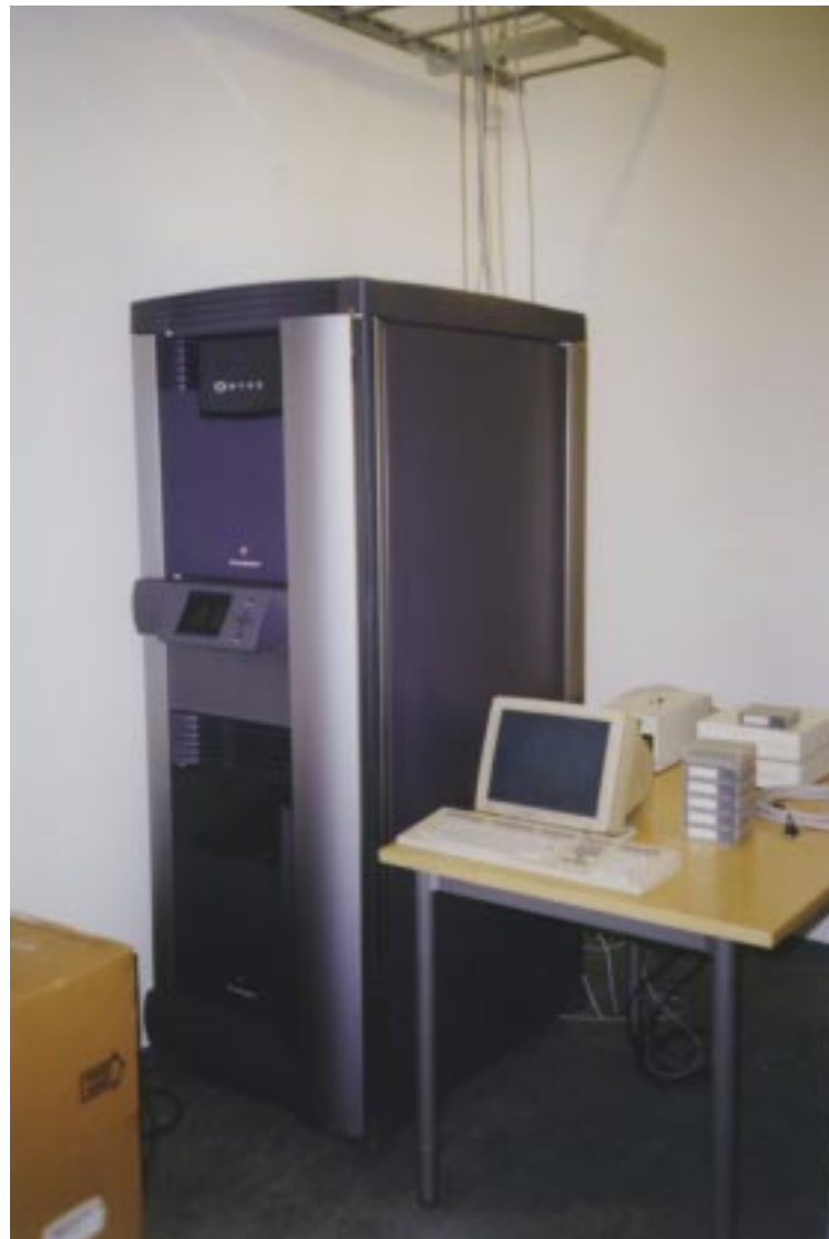
Figure 43: The Onyx2 installed. On the right side of the Onyx, an ASCII console for controlling the computer in case of problems, and the backup devices.
