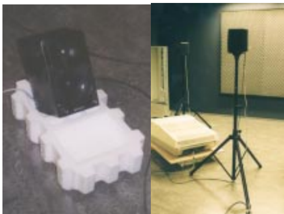
Figure 52: The floor and head-level mountings of the loudspeakers.
