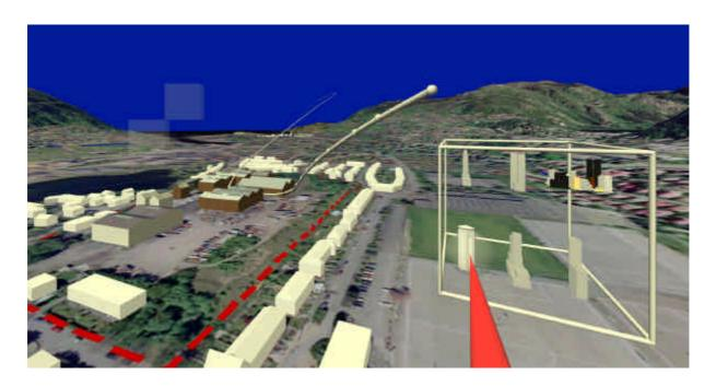
Figure 1: A model of the Bergen area with buildings at Kronstad (near) and downtown (far). To the right is a menu for importing buildings. Also shown is a spline with control points representing an editable flight path.
