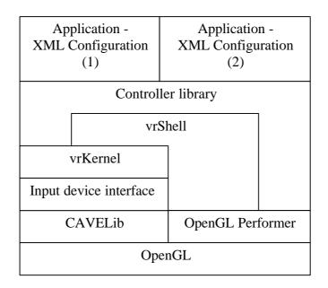
Figure 2: System architecture and dependence of main components
